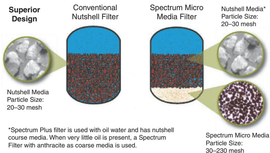
Fig. 1—Conventional nutshell filter compared with Spectrum micro media filter.
