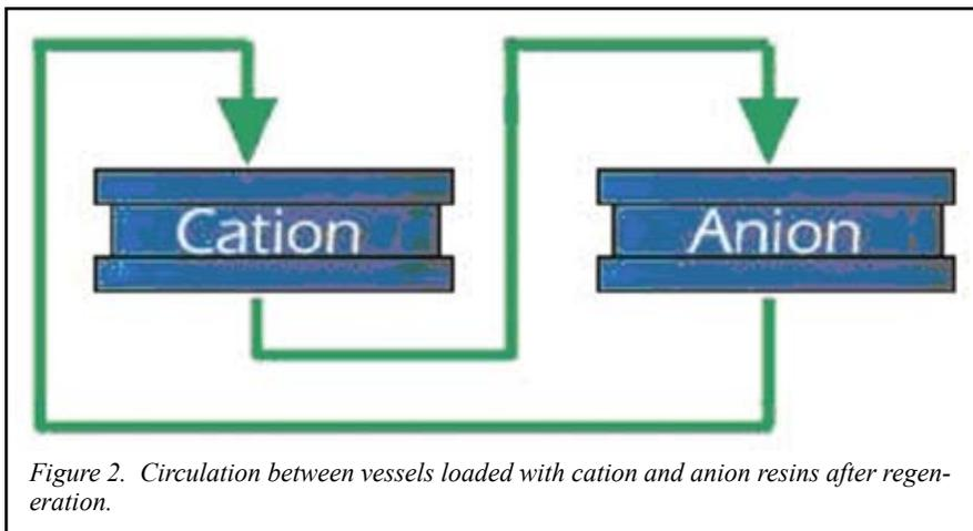
Figure 2. Circulation between vessels loaded with cation and anion resins after regeneration.
