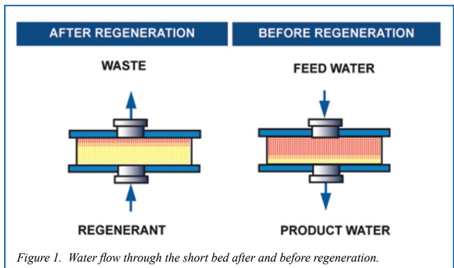
Figure 1. Water flow through the short bed after and before regeneration.
